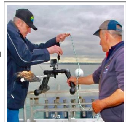
This baited remote underwater video (BRUV) unit is used to capture footage of fish species.
